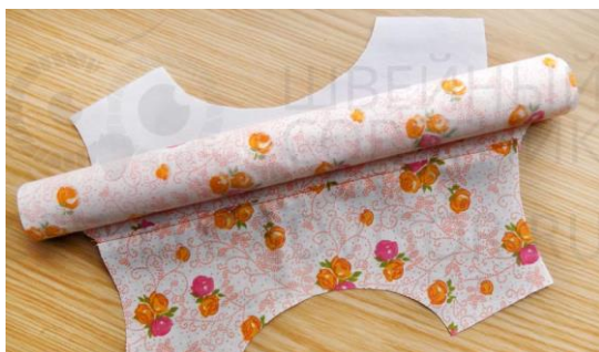
92-rasm: Koketkani orqa qismini rulondek aylantirish
