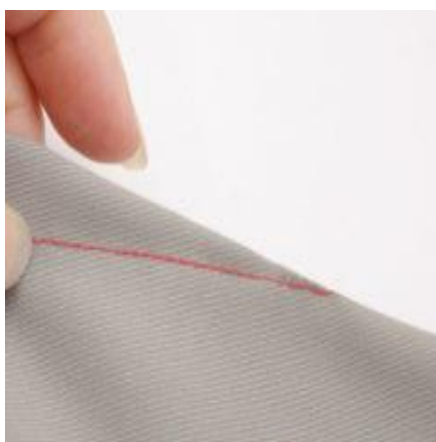
57-rasm: Yupqa shifondan matolarga vitochka tikish
